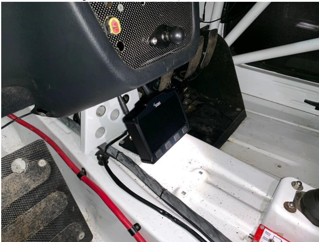
Figure 2. The WRC tracking unit mounted onto the 25mm rubber ball mount and connected through the RallySafe connector
